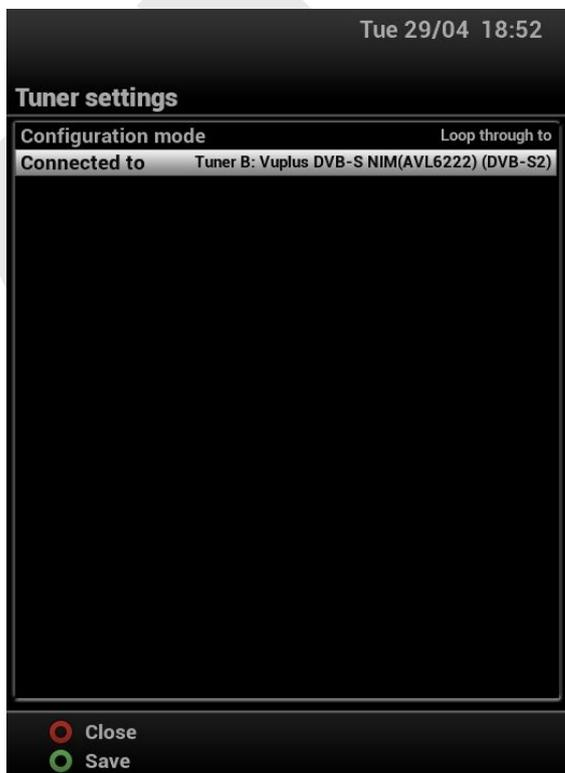
NB1: some tuners require a physical cable from 'LNB-out' of the other tuner to 'LNB-in' of this tuner; whereas other tuners have an internal loopthrough (so this setting will actually make the connection).
